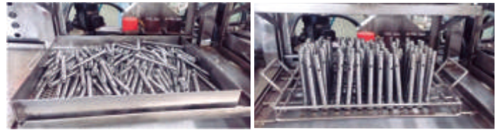
Quality improvement: Jig basket used for vertical washing of seat pipes, reducing metal to metal contact
