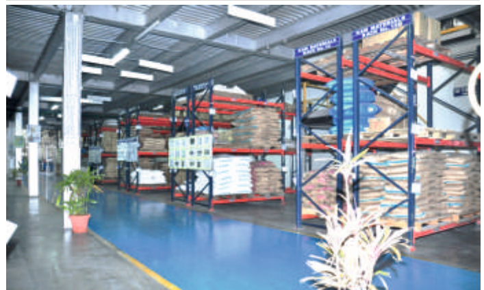
Raw material storage system (Computerized with bar code system)
