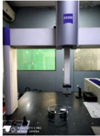
Zeiss CMM Machine for Coordinates measurement for Gears of Class 1 as well
