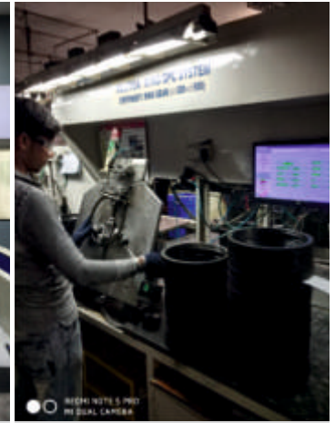
Multi-gauging Equipment for deskilling operator and error-proofing
