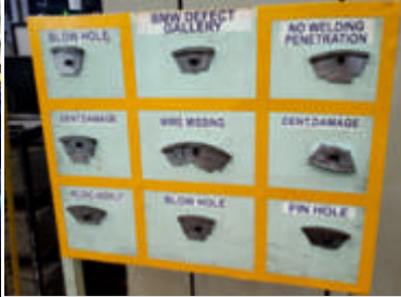
BMW Defect Gallery for Operator training
