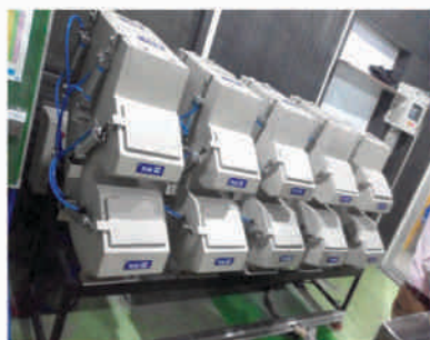
Chemical Weighing System
