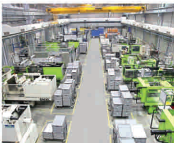
Moulding shop equipped with 18 Nos molding machines ranging from 80 Ton to 1360 Ton.
