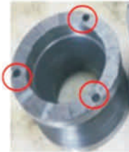
Required 3 bolts to tightened the Hobbing Fixture Result in more time to change set up
