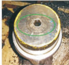
Required Only One Allen Bolt to tightened the Auto Loading Locator Result : Save Set Up time
