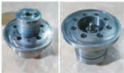
Required 3 bolts to tightened the Auto Loading Locator Result in more time to change set up
